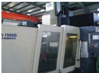
HTM-1500G Portal-type Pentahedron CNC(X/Y/Z) 2000mm/1500mm/700mm
