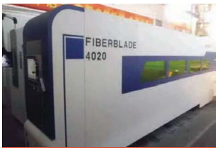
Laser cutting machine Operating space (X/Y/Z)4020mm/2020mm/300mm
