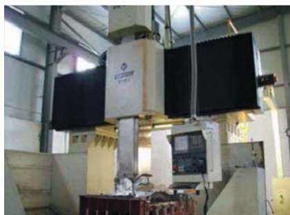
HTM-25G × 40 Portal-type Pentahedron CNC (X/Y/Z) 2500mm/2700MM+215mm/1000mm
