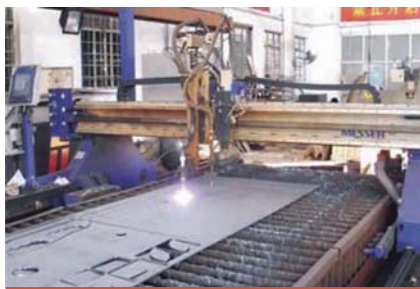
MESSER Fine plasma cutting machine (X/Y) 4000mm/12000mm
