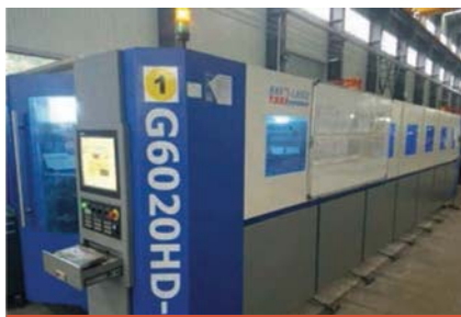
Laser cutting machine Operating space (X/Y/Z)6030mm/2020mm/300mm
