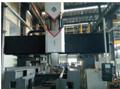
HTM-25G × 40 Portal-type Pentahedron CNC (X/Y/Z) 2500mm/2700MM+215mm/1000mm
