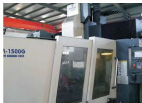
HTM-1500G Portal-type Pentahedron CNC(X/Y/Z) 2000mm/1500mm/700mm
