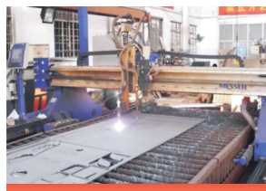
MESSER Fine plasma cutting machine (X/Y) 4000mm/12000mm
