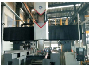
HTM-25G X 40 Portal-type Pentahedron CNC (X/Y/Z) 2500mm/2700MM+215mm/1000mm
