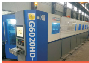
Laser cutting machine Operating space (X/Y/Z)6030mm/2020mm/300mm
