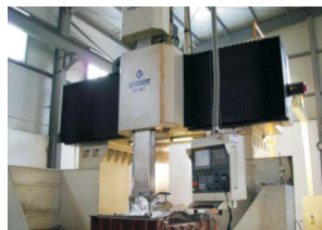
HTM-25G X 40 Portal-type Pentahedron CNC (X/Y/Z) 2500mm/2700MM+215mm/1000mm
