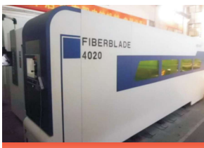
Laser cutting machine Operating space (X/Y/Z)4020mm/2020mm/300mm
